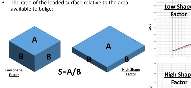
• Rubber deforms, it does not compress
